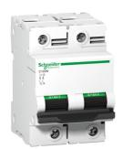
Miniature circuit breaker (MCB), Acti9 C120N, 2P, 100A, D curve, 10000A (IEC/EN 60898-1), 10kA (IEC/EN 60947-2)
