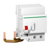
Vigi C120 - earth leakage add-on block - 2P - 30 mA - class AC
