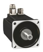
servo motor BMH, Lexium 32, 6.2Nm, 6000rpm, keyed shaft, with brake, IP54, 128bit encoder, straight
