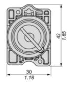
(e) Clamping thickness: 1 to 6 mm / 0.04 to 0.24 in.
