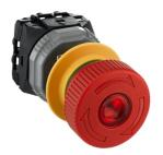
Illuminated emergency stop push button, Harmony XB5, plastic, red, mushroom 40mm, 22mm, trigger latching turn to release, 24V DC, 1NO 2NC
