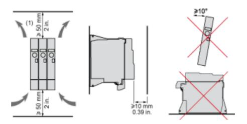
(1) Minimum value corresponding to thermal constraints.
