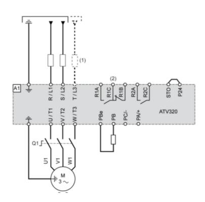
(1) Line choke (if used)(2) Fault relay contacts, for remote signaling of drive status
