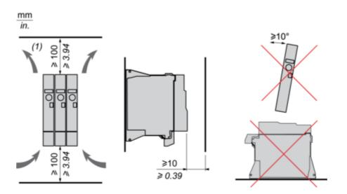
(1) Minimum value corresponding to thermal constraints.
