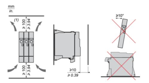
(1) Minimum value corresponding to thermal constraints.
