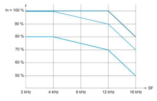
40 °C (104 °F) - Mounting type A, B and C 50 °C (122 °F) - Mounting type A, B and C 60 °C (140 °F) - Mounting type B and C In : Nominal Drive Current
