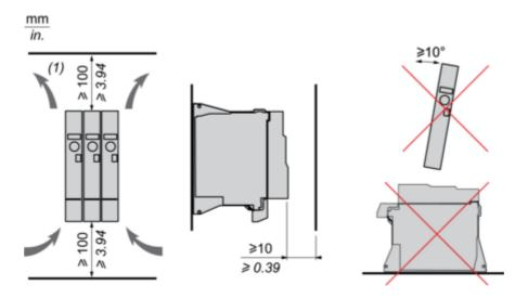
(1) Minimum value corresponding to thermal constraints.
