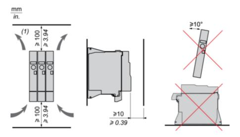
(1) Minimum value corresponding to thermal constraints.
