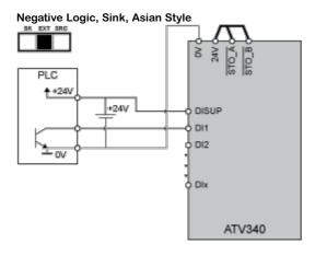
Digital Inputs: Internal supply Negative Logic, Sink, Asian Style
