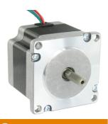
2-phase stepper motor - 1.69 N.m - shaft Ø6.35 mm - L=76mm - without brake - 3A
