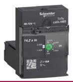
Standard control unit, TeSys U, 0.35-1.4A, 3P motors, magnetic protection, coil 48-72V AC/DC
