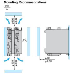
LXM32•U45M2, •U90M2 and LXM32•U60N4 servo drives are cooled by natural convection. LXM32•D18M2, •D30M2, LXM32 •D12N4, •D18N4, •D30N4 and •D72N4servo drives have an integrated fan. When installing the servo drive in the enclosure, follow the instructions below with regard to the temperature and protection index:
