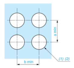
(1) Diameter on finished panel or support (2) Ø30 mm recommended / Ø1.2 in. recommended
