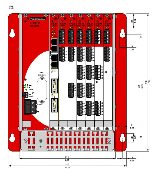
Max. module depth including screw terminals for the power supply: 239 mm/ 9.21 in.
