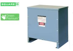
Low voltage transformer, non ventilated dry type, 3 phase, 112.5kVA, 480V primary, 208Y/ 120V secondary, Type 3R
