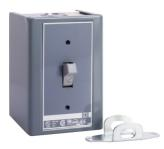
Switch, manual, 30A, 2 pole, 3 HP at 575 VAC, single phase, toggle operated, no indicator, NEMA 1 jumbo enclosure
