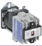
NEMA Control Relay, Type X, utility, 10A resistive at 600 VAC, 12 normally open contacts, 48 VDC coil
