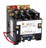
NEMA Contactor, Type S, nonreversing, Size 0, 18A, 5 HP at 575 VAC, 3 phase, up to 100 kA, 5 pole, 480 VAC coil, open
