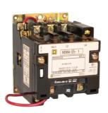
NEMA Contactor, Type S, nonreversing, Size 1, 27A, 10 HP at 575 VAC, 3 phase, up to 100 kA, 5 pole, 120 VAC coil, open
