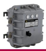
NEMA Contactor, Type S, nonreversing, Size 1, 27A, 10 HP at 575 VAC, 3 phase, 3 pole, 120VAC coil, NEMA7/9
