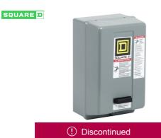
NEMA Motor Starter, Type S, nonreversing, Size 00, 9A, 1 HP at 230 VAC, 5 kA SCCR, 1 phase, 2 pole, melting alloy, 120 VAC coil, NEMA 1
