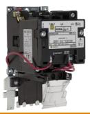
NEMA Motor Starter, Type S, nonreversing, Size 1, 27A, 10 HP at 460 VAC, up to 65 kA SCCR, 3 phase, 3 pole, bimetal, 240 VAC coil, open
