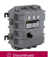
NEMA Motor Starter, Type S, nonreversing, Size 1, 27A, 3 HP at 230 VAC, 1 phase, 2 pole, melting alloy, 240 VAC coil, NEMA 7/9
