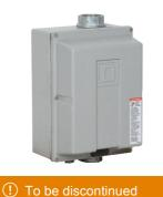
NEMA Motor Starter, Type S, nonreversing, Size 2, 45A, 25 HP at 460 VAC, 5 kA SCCR, 3 phase, 3 pole, melting alloy, 120 VAC coil, NEMA 4X
