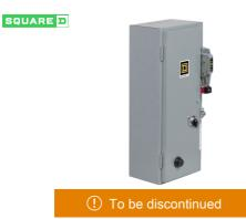
NEMA Combination Starter, Type S, 30A fusible disconnect, Size 1, 27A, 5 HP at 240 VAC polyphase, 120 VAC coil, NEMA 1
