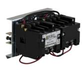
NEMA Contactor, Type S, reversing, horizontal, Size 00, 9A, 2 HP at 575 VAC, 3 phase, up to 100 kA, 3 pole, 208 VAC coil, open style
