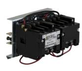
NEMA Contactor, Type S, reversing, vertical, Size 1, 27A, 10 HP at 575 VAC, 3 phase, up to 100 kA, 3 pole, 24 VAC coil, open style
