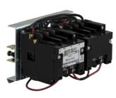
NEMA Contactor, Type S, reversing, horizontal, Size 1, 27A, 10 HP at 575 VAC, 3 phase, up to 100 kA, 3 pole, 600 VAC coil, open style
