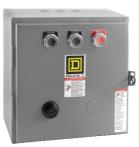
NEMA Starter, Type S, reversing, horizontal, Size 00, 9A, 2 HP at 575 VAC, up to 100 kA SCCR, 3 phase, 3 pole, Motor Logic SSOLR, 240 VAC coil, NEMA 1
