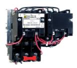
NEMA Starter, Type S, reversing, horizontal, Size 00, 9A, 2 HP at 575 VAC, 5 kA SSCR, 3 phase, 3 pole, melting alloy overload, 480 VAC coil, open
