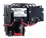
NEMA Starter, Type S, reversing, horizontal, Size 0, 18A, 2 HP at 230 VAC, 5 kA SSCR, 1 phase, 3 pole, melting alloy overload, 120 VAC coil, open
