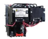
NEMA Starter, Type S, reversing, horizontal, Size 0, 18A, 5 HP at 575 VAC, 5 kA SSCR, 3 phase, 3 pole, melting alloy overload, 24 VAC coil, open
