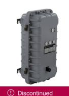
NEMA Starter, Type S, reversing, horizontal, Size 0, 18A, 5 HP at 575 VAC, 3 phase, 3 pole, melting alloy overload, 120 VAC coil, NEMA 7/9
