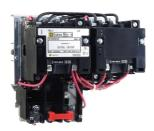
NEMA Starter, Type S, reversing, horizontal, Size 1, 27A, 10HP at 575VAC, up to 100kA SCCR, 3 phase, 3 pole, Motor Logic SSOLR, 120V coil, NEMA 1
