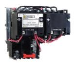
NEMA Starter, Type S, reversing, horizontal, Size 1, 27A, 10 HP at 575 VAC, up to 100 kA SCCR, 3 phase, 3 pole, Motor Logic SSOLR, 240 V coil, NEMA 1
