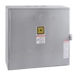
Contactor, Type L, multipole lighting, electrically held, 30A, 10 pole, 600 V, 110/120 VAC 50/60 Hz coil, NEMA 1
