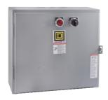
Contactor, Type L, multipole lighting, electrically held, 30A, 12 pole, 600 V, 277 VAC 60 Hz coil, NEMA 1, +option
