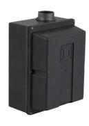
Contactor, Type L, multipole lighting, mechanically held, 30A, 4 pole, 600 V, 277 VAC 60 Hz coil, NEMA 4/4X
