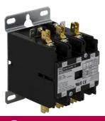
Contactor, Definite Purpose, 30A, 3 pole, 20 HP at 575 VAC, 3 phase, 24/24 VAC 50/60 Hz coil, open, CU/AL box lugs
