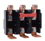
Overload Relay, Type S, melting alloy, replacement overload, NEMA size 3, 5 pole, 3 phase, 90A, 600VAC
