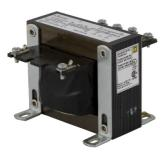
Transformer, EO, industrial control, 75VA, 1 phase, 240x480V primary, 120V secondary, 80C rise
