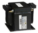
Transformer, Type T, industrial control, 1000VA, 1 phase, 277V primary, 120V secondary, 115C rise
