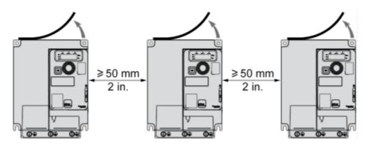
For Operation at Ambient Temperature Above 50  $^{\circ}\text{C}$  (122  $^{\circ}\text{F})$
