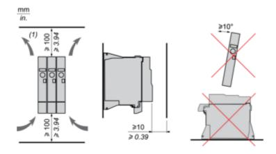
(1) Minimum value corresponding to thermal constraints.
