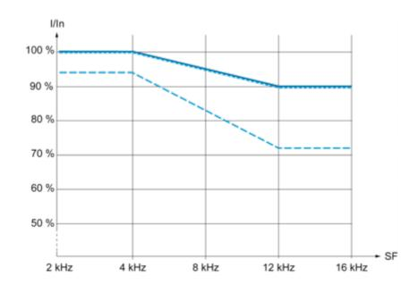
40 °C (104 °F) - Mounting type A, B and C 50 °C (122 °F) - Mounting type C 60 °C (140 °F) - Mounting type C
