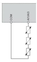
It is possible to connect either 1 or 3 sensors on terminals Al1/Al3.
