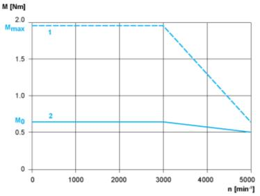
Servo Motor with LXM28AU02••• Servo Drive
